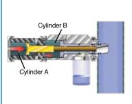
Cylinders A and B advance plunger; annulus is closed
