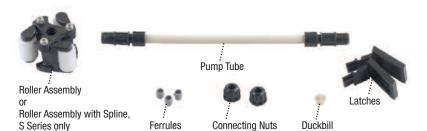
The Classic, SVP, M128 and S series are manufactured with the patent pending QuickPro® pump head. The QuickPro® contains a collapsible roller assembly and the housing is attached by latches instead of screws.
