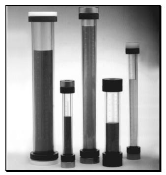
Griffco Borosilicate Glass Calibration Cylinders are designed to enhance the performance of chemical feed systems by providing a verification of the flow rate of the chemical feed pump. Constructed of borosilicate glass and a choice of 7 end cap materials, (PVC, CPVC, PP, PTFE, PVDF, 316 SS, A20) these cylinders are suitable for use with most chemicals. 9 sizes; 30 mL, 100 mL, 200 mL, 500 mL, 1000 mL, 2000 mL, 4000 mL, 10 L, 20 L.
